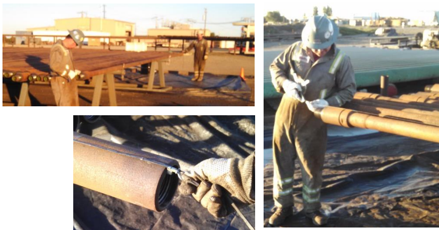
Figure 67: Drill pipe strapping in defining drill pipe length
