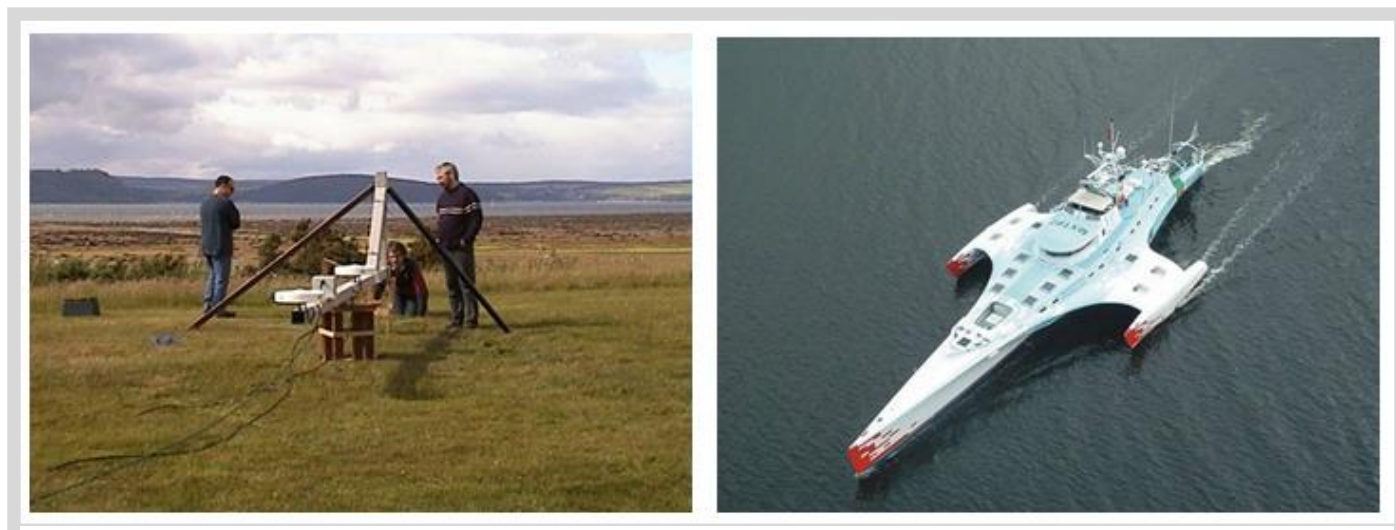
Figure 41: Calibrating a marine observation frame on land & using a non-magnetic vessel for marine surveying
