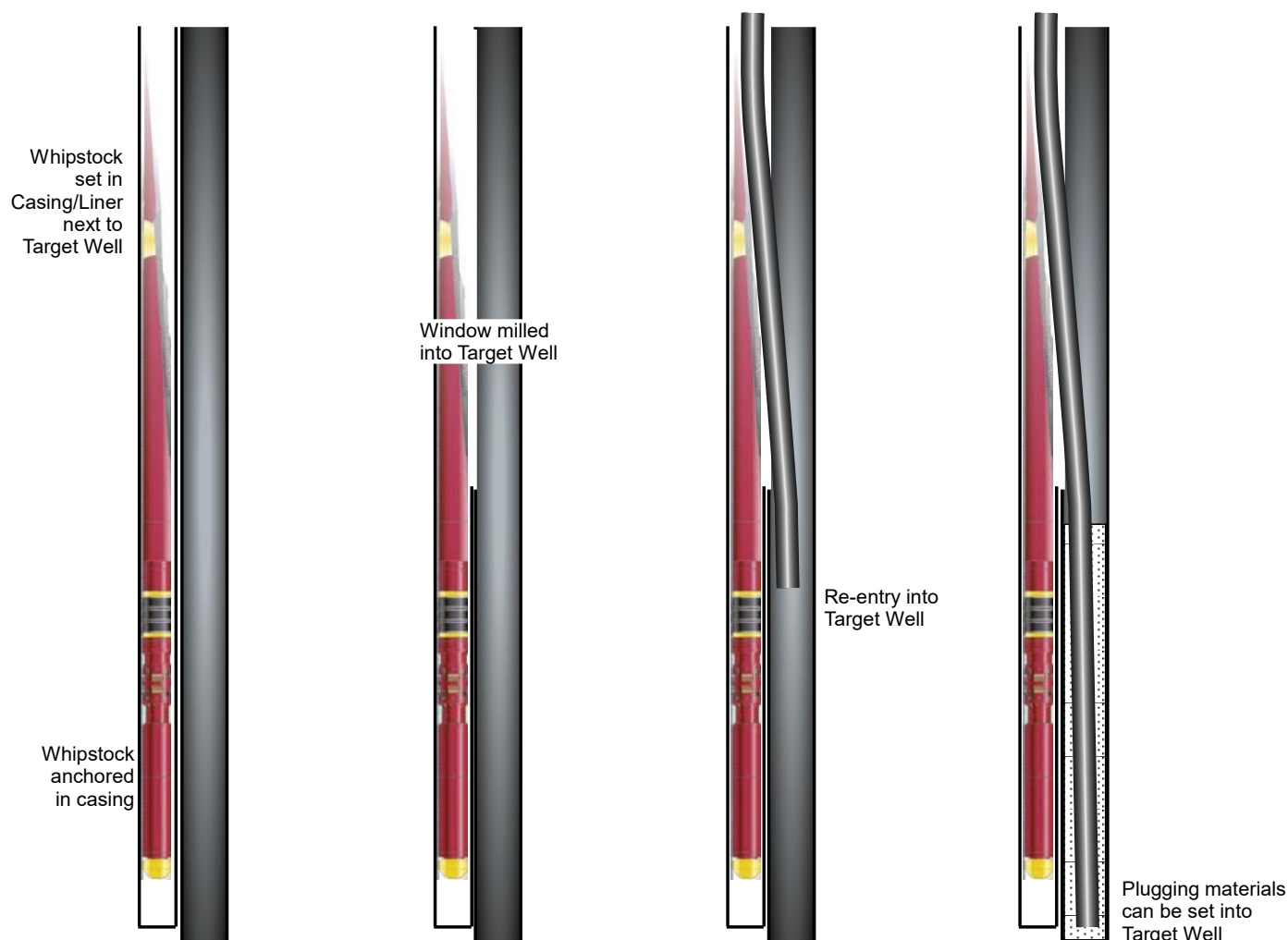
Figure 64: Cased Hole Whipstock Milling Method Concept
